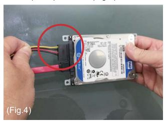
4. Connect the SATA Power cable with HDD. 5. Attach the thermal pad on the HDD (Fig.4)
