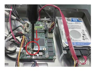
14. Push the mSATA down to the motherboard Fasten mSATA with the (M2\*6) screw.(Fig.14)
