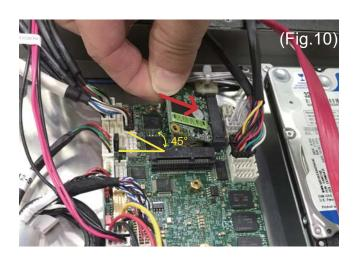
10. Install the mSATA into the connector slot at a 45 degree angle. (Fig.10)
