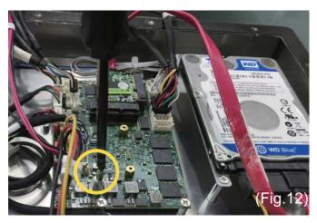
12. Unscrew the(M2\*6) screw from the screw thread on motherboard. (Fig.12)
